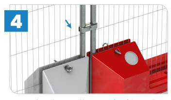
Use a coupler at the top and bottom section of the panel to secure in place.
